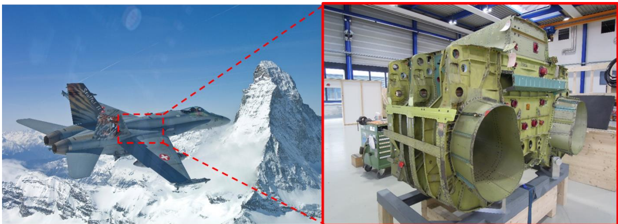
Figure 8: The FTS3 centre barrel test article comprising three Ti-6Al-4V wing carry-through bulkheads.
