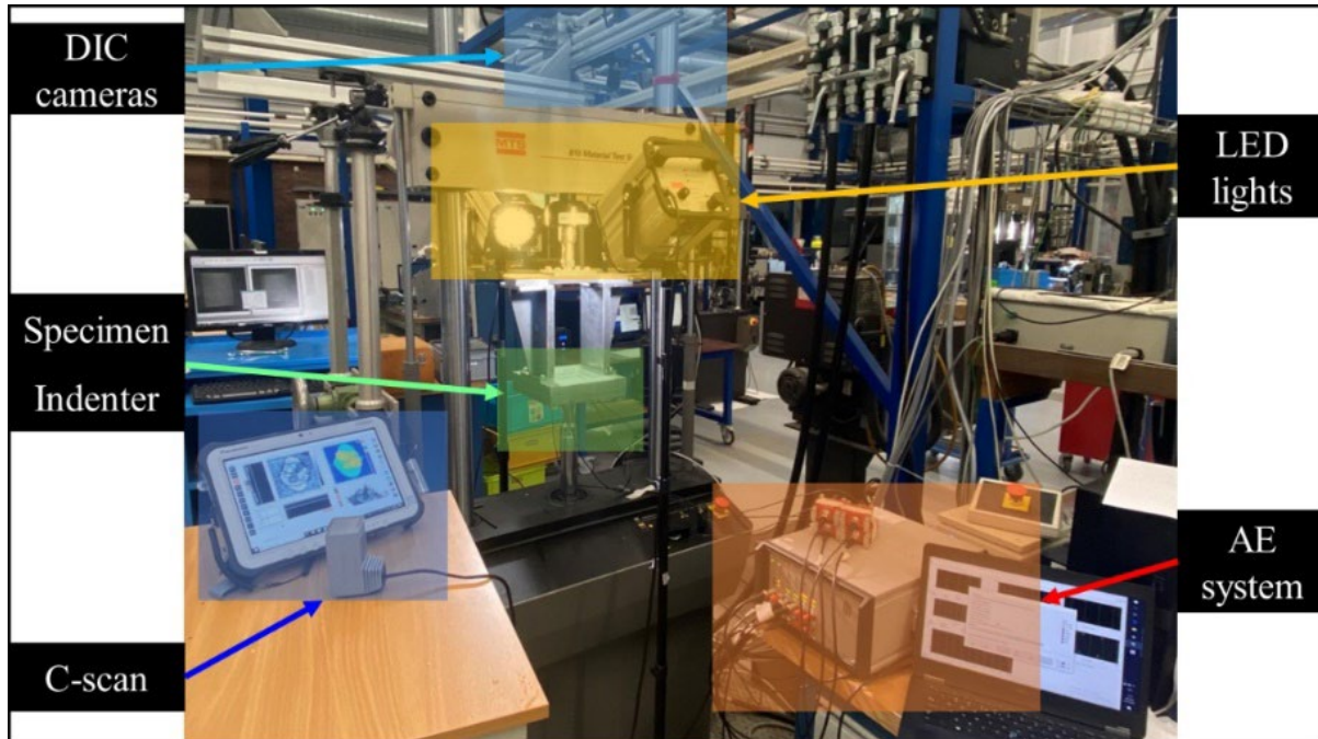
Figure 2: Illustration of the specimen geometry and basic setup.
