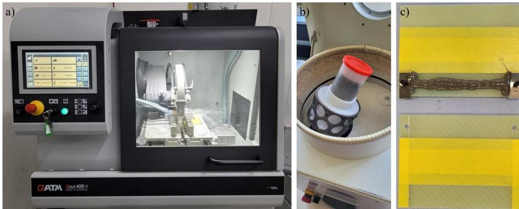
Figure 1. Fabrication process of the SLS joints: a) cutting of the plates, b) mixing of the adhesive system and c) bonding process.
