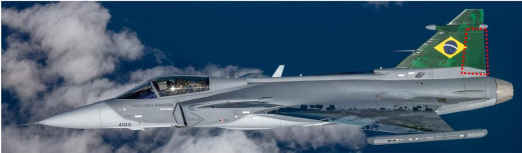
Figure 1: Gripen 39E with the rudder highlighted with a red dotted line. Copyright SAAB AB, photo Linus Svensson.
