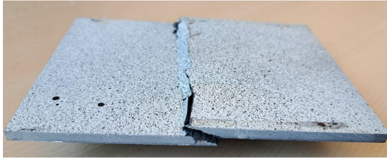
Figure 4: Failed specimen after CAI fatigue test.
