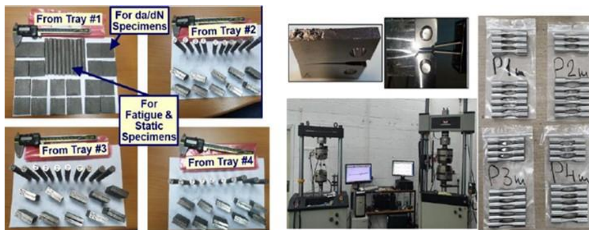
Figure 2: AM tested specimens, for the four print parameters sets and testing machines.
