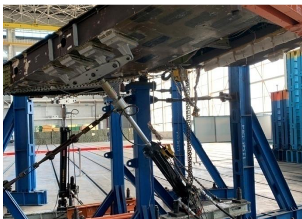
Fig. 6 Photo of the verification test of the tension/shear block-levers system.
