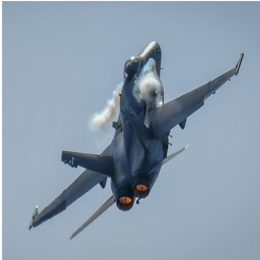
Figure 1. High-energy vortices generated by the inner wing leading edge extensions (LEX) resulting regions of low pressure that condenses the water vapor of the air (left figure: courtesy of the FINAF) and induce severe cyclic loading to the downstream structure, like Vertical Tails, by exciting the resonance frequencies of the empennage (right figure, edited from Ref. [1]).
