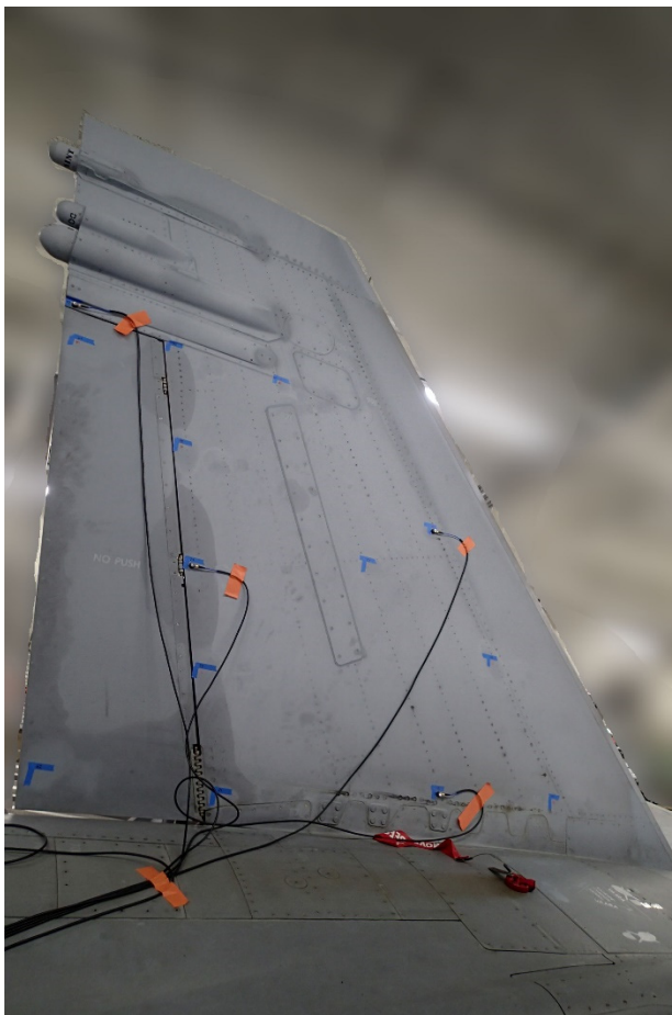
Figure 5. Some of the measurement locations on the LH VT (left) and excitation location of impact testing for LH VT (Tip Rib/Spar joint) (right).
