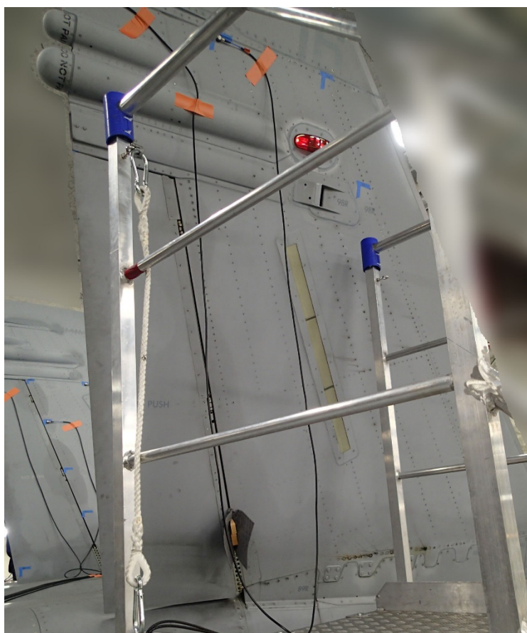
Figure 3. A general view of measurement arrangements. The RH rudder was locked by a soft wedge as shown in the photo.
