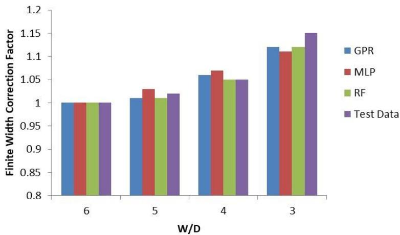
Figure 4: Predictions vs. Test data
