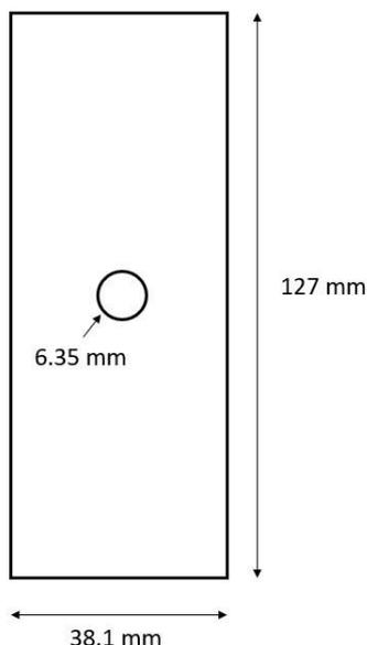
Figure 1: Open hole test specimen dimensions (W/D = 6.0)
