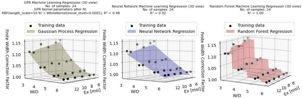
Figure 2: Regression surfaces to obtain finite width correction factors using the GPR (left), MLP (middle) and RF (right) algorithms
