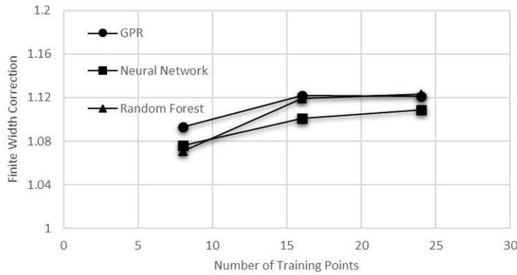
Figure 3: Sensitivity of the predicted finite width correction factors with respect to the number of training points ( $W/D = 3.1, [02, 90, \pm 452]$ )
