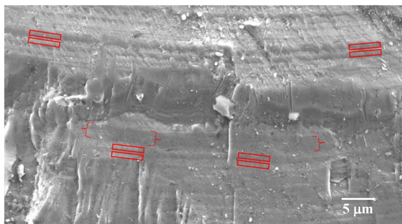
Figure 2: Ongoing QF using SEM with magnification of 1000 x [10]. Aluminium specimen (7075-T76) was fatigue tested with BOS2 spectrum, and some traced striations are pre-marked.
