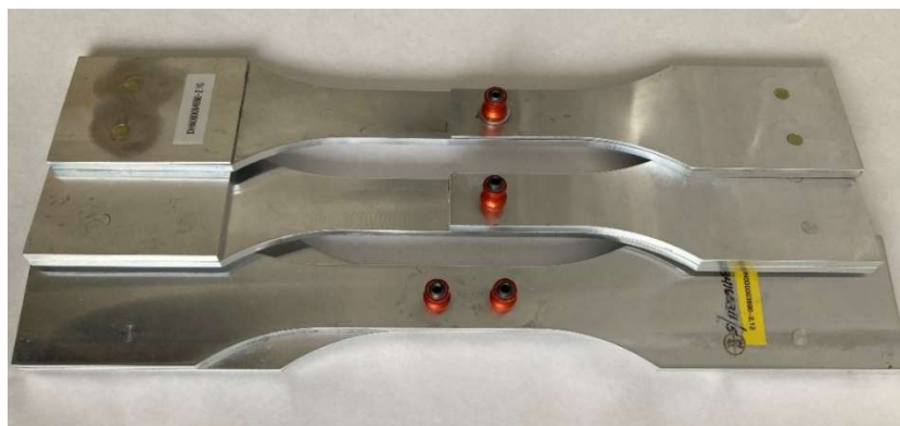
Figure 7: Three aluminium 7075-T76 ESDU specimen types to be tested [11]. Types counting from top: MLT1, MLT2, and LLT.
