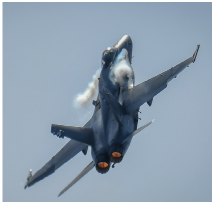
Figure 1. High-energy vortices generated by the inner wing leading edge extensions resulting regions of very low pressure that condenses the water vapor of the air (left figure: courtesy of the FINAF) and induce severe cyclic loading to the downstream structure, like Vertical Tails, by exciting the resonance frequencies of the empennage (right figure, edited from Ref. [1]).
