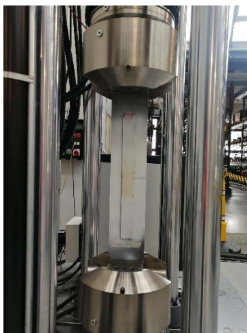
Figure 4. Fatigue test setup.
