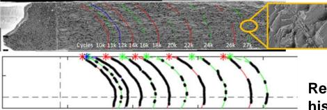
Reconstruction of crack growth history via marker band location
