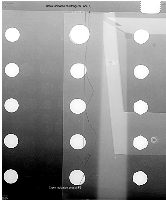
Radiograph of Cracked Space Shuttle External Tank Stringer
