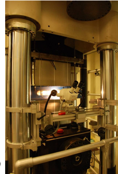
Servo-hydraulic machine: f \leq 5 Hz, R_F = 0.1
