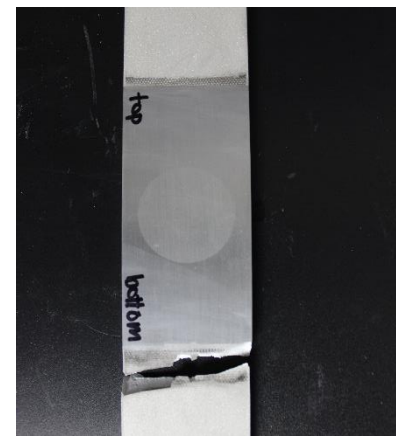
Grip Failure R= 0.1 N= 38,524 cycles
