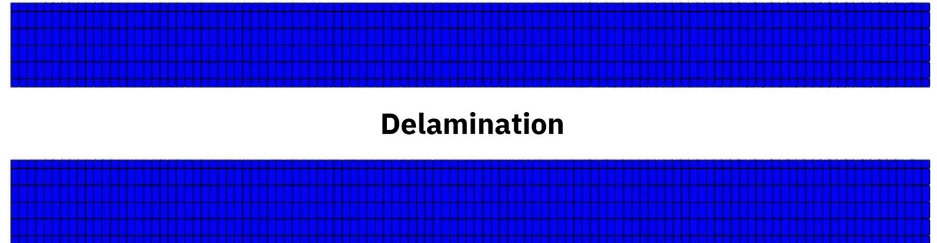
Results confirm Bethelot's findings: the crack density evolution cannot be captured without including delamination
