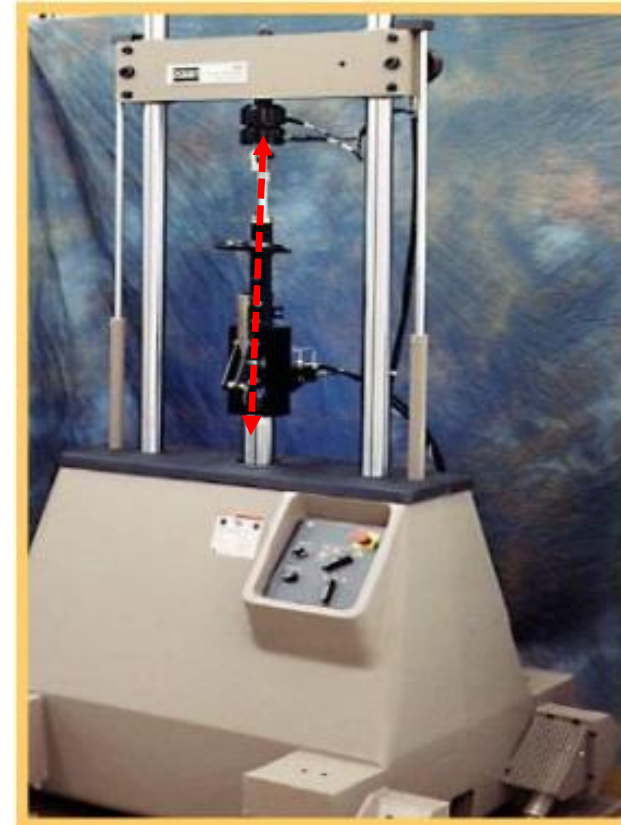
Test Frame With Specimen (physical Substructure)
