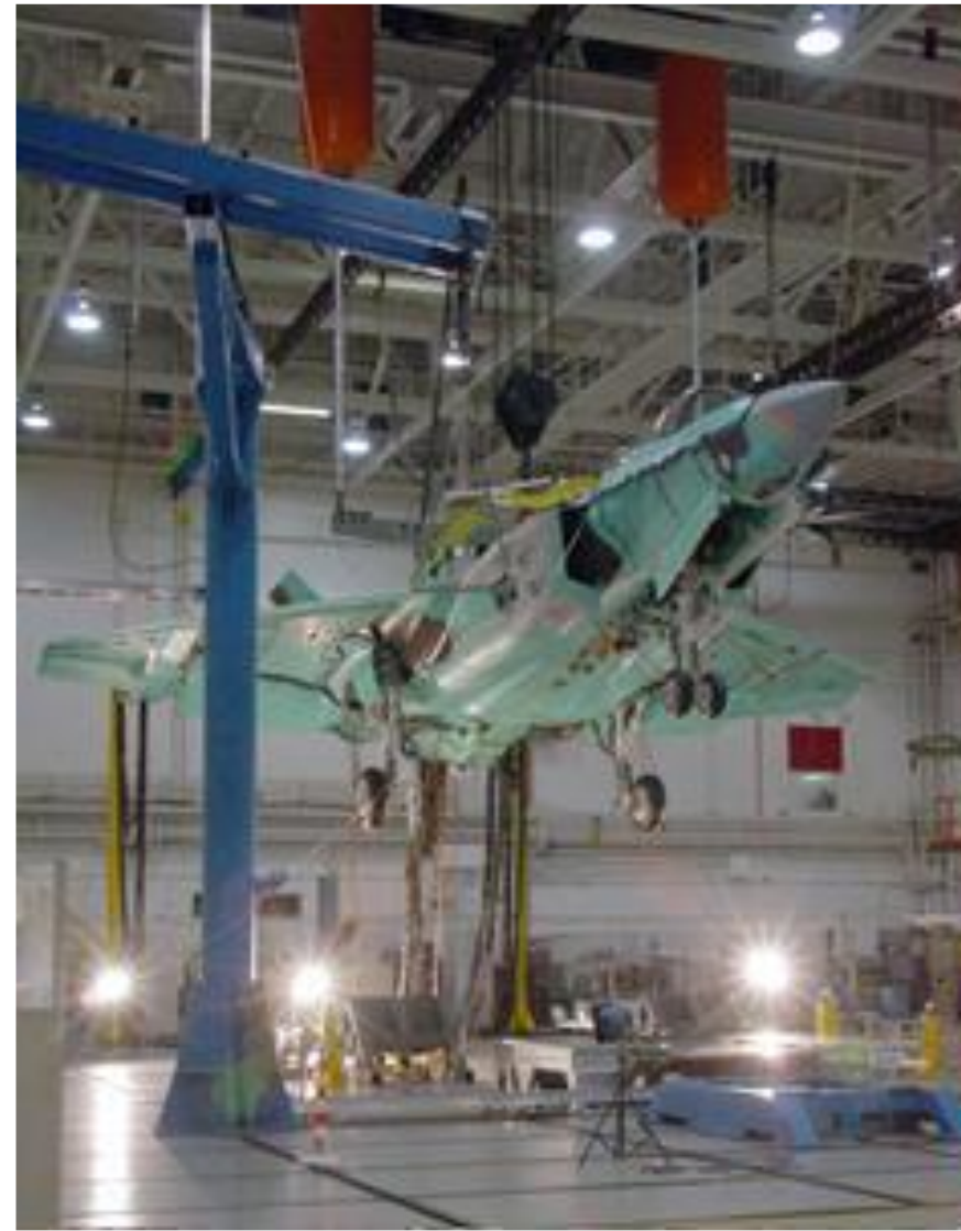
Naval version of F-35 aircraft tests in multiple landing scenarios.
