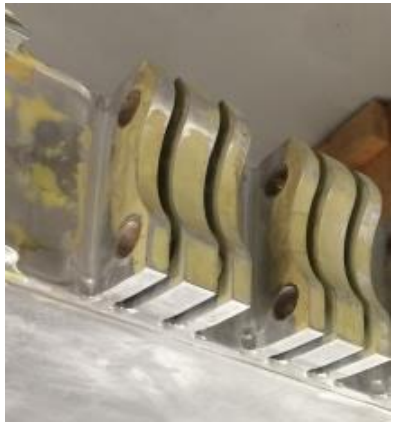
CF-188 inboard leading edge flap lugs with modifications
