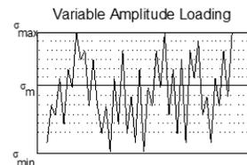
Design analysis with crack growth analysis
