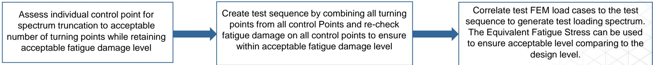
A control points study on critical fatigue or DT locations and major loading point locations across the test structure is performed in order to determine a simplified spectrum and applied loads while retaining a representative level of fatigue damage within the structure. Control Points Selection criteria include:
