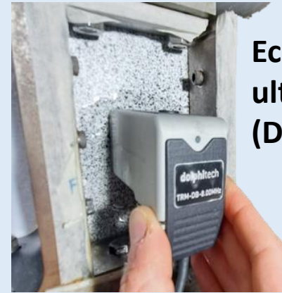
Through thickness transmission ultrasound scan
