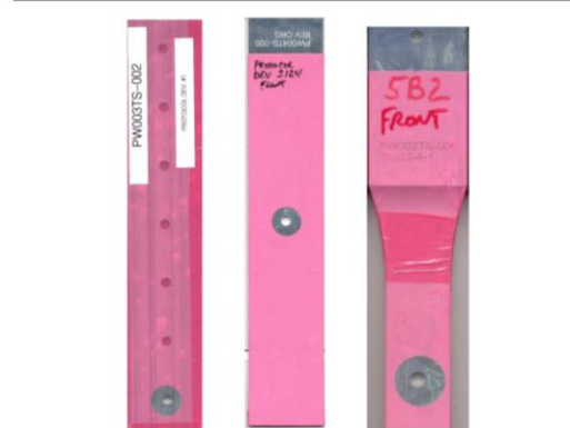
Figure 6 (L) Representative image of a multihole protocol development specimen taped off to expose one bore hole for corrosion testing; (C) Representative image of a single hole protocol development specimen taped off to expose one bore hole for corrosion testing; (R) Representative image of a dog bone fatigue test specimen taped off to expose the bore hole for corrosion testing (note: only top 2/3 of dog bone visible in scan image, although entire dog bone was taped).
