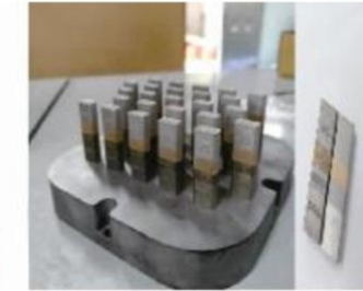
Graded functional material (SLM), Yang, 2019
